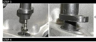
Slide the bent end of the link through the attachment hole at the end of the TV cable. Gently pull on the opposite end of the TV cable (carburetor/fuel injection end) of the TV cable while feeding the transmission end of the cable housing down into the transmission seal. Be sure the wire link doesn't slip out while performing this procedure.
