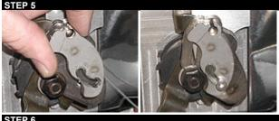
Align the roll pins on the back side of the cam into the slots on the linkage adapter plate. Once the cam is indexed correctly, install the 8/32" cap screw and tighten using the provided 9/64" Allen wrench. Use cautionI not to over tighten this small screw.
