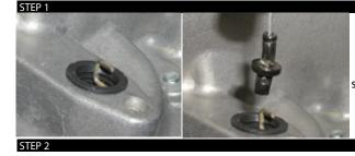
The TV cable is connected to the passenger side of Th-2004R and Th-700R4 transmissions at the locations shown in the above pictures. Same side as your dipstick. The picture at the far left show s the wire link and the TV cable to case seal. This seal must be placed into the transmission before installation, not onto the end of the TV cable housing! The wire link will be inserted into the hole of the connector at the transmission end of the TV cable. (See closest picture at left)
