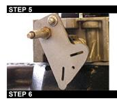
Reinstall the throttle cable stud on to the linkage.
