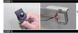
Insert the TV cable into the base plate bracket until you hear it click into position. To do this, match the index guide on the TV cable housing, with the notch in the base plate bracket (red circles in pictures at left). The TV cable will not go in any other way.
