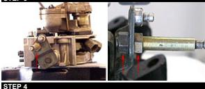
In order to install the back plate, you will need to temporarily remove the throttle cable stud from the linkage. Once you have this stud removed, place it aside as you will be putting it back on.
