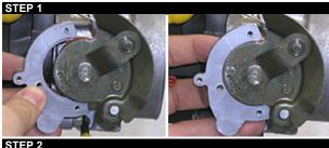
Locate the back plate/spacer plate piece in the TV Made EZ kit (far left picture). Notice that this part has a lipped section on the inside radius. Using this lip as a guide, place this adapter onto the LS-1 linkage from the back side as shown in the picture near left. This part is designed to fit snuggly so a light amount of force may be needed for installation.
