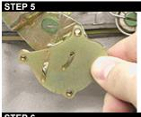
Position the front face plate of the linkage adapter over the linkage as shown in the picture on the left. Now turn the face plate until the four bolt holes line up with the back plate section installed in the previous step.
