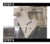
Reinstall the throttle cable stud on to the linkage.
