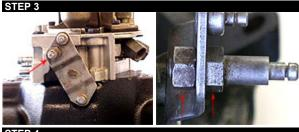
In order to install the back plate, you will need to temporarily remove the throttle cable stud from the linkage. Once you have this stud removed, place it aside as you will be putting it back on.
