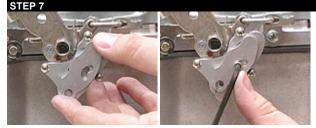
Align the roll pins on the back side of the cam into the slots on the linkage adapter face plate. Once the cam is indexed correctly, install the 8/32" cap screw and tighten using the provided 9/64" Allen wrench. Again be careful not to over tighten this small screw.
