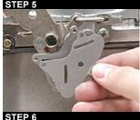
Position the front face plate of the linkage adapter over the linkage as shown in the picture on the left. When correctly positioned, this face plate will index over the extruded (raised area) hole on the linkage. Once indexed over the extruded hole, simply turn the face plate until the four bolt holes line up with the back plate section installed in the previous step.
