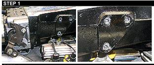
Remove the old throttle cable bracket from the manifold. Be sure to save the bolts that you remove as you will be reusing them.
