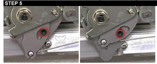
You are ready to perform your test drive! We recommend the pressure gauge remain hooked up during all test driving. Pay attention to the reactions caused by the TV system, it is very educational. During the test driving we also recommend Allen wrench supplied in the TV Made EZ kit that fits the cap screw shown within the red circles at left. Start with the cam in the lower position (far left picture), perform a test drive while making mental notes of the shift timing and feel characteristics.
