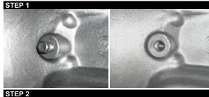
The pressure gauge must be connected to the transmission at the location shown above. This is a direct fluid passage to the transmissions internal hydraulic pump. This installation will be done while the engine not running. Testing will be done with the engine running. To hook up the gauge, locate the 1/8" plug on the "Driver Side" of the transmissions bell housing as shown in the above pictures; unscrew the plug from the transmission.
