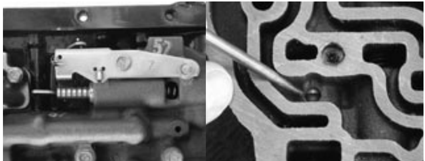
The throttle-valve feed orifice (pointer, right photo) is the only load communication to the transmission. The throttle valve controls the feed orifice and when properly adjusted, it sits right at the edge of the orifice eagerly waiting to uncover it, boosting pressure as the throttle opens and the engine makes more power.
