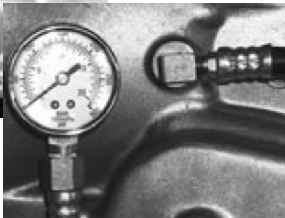
By connecting a pressure gauge to the transmission's pressure port (arrow), the function of the throttle valve can be monitored. The trans should produce 55-65 psi at idle and should immediately rise with any movement of the throttle-valve cable.
