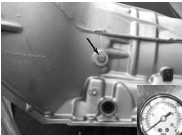
By connecting a pressure gauge to the transmission's pressure port (arrow), the function of the throttle valve can be monitored. The trans should produce 55-65 psi at idle and should immediately rise with any movement of the throttle-valve cable.
