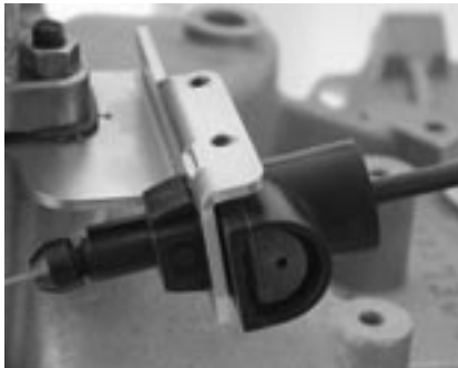
The GM self-adjusting cable uses a ratcheting action to tighten itself.
