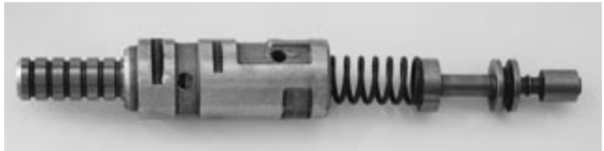
The throttle valve is responsible for the life of your transmission and the quality of the shifts.
