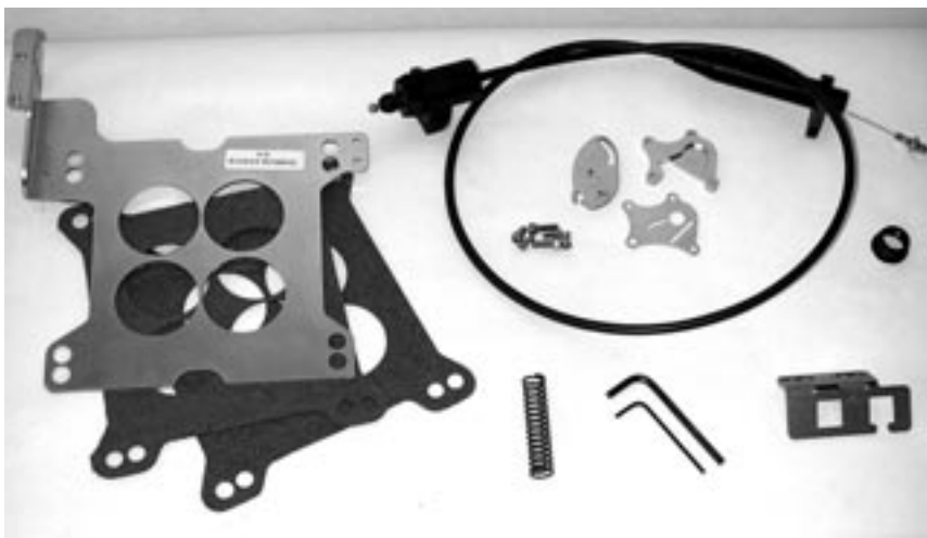
Bowtie Overdrives offers complete throttle-valve-system kits for 14 different applications. Retailing for around $110, the kit features a new GM TV cable, an adjustable cam system, a TV cable baseplate, all necessary gaskets and hardware, a matched throttle-valve spring, and the Allen wrenches necessary to adjust the shift quality of your trans. An extra $14 will get you a steel-braided TV cable.
